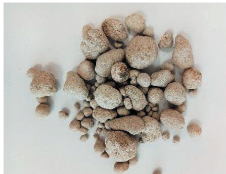
Fig. 1. Lightweight artificial aggregate produced in autoclaving process.
